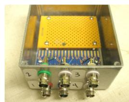
Figure 7. DUT in sample box used for Van der Pauw measurements
