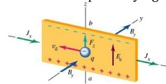
Figure 5. Charge accumulation due to Hall effect.
