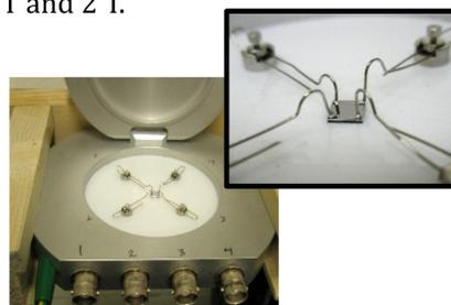
Figure 9. DUT prepared for Hall measurements with closeup of sample
