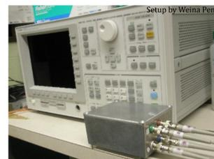
Figure 8. DUT connected to semiconductor parameter analyzer for Van der Pauw measurements
