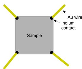
Figure 6. Contact arrangement for a device under test (DUT)
