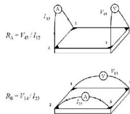
Figure 4. Configuration for Van der Pauw method.
