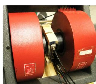
Figure 10. DUT positioned in magnet for Hall measurements
